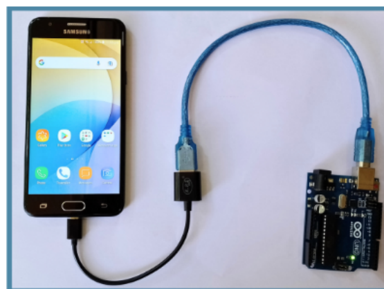
Figure 2. Arduino uno microcontroller connected to a Mobile phone through an OTG cable and an USB port
