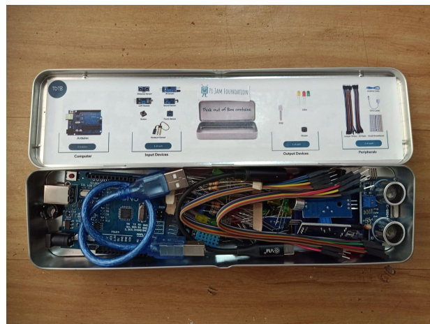
Figure 1. Think out of the box kit containing an arduino uno, connecting wires, breadboard and a variety of sensors and actuators
